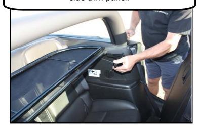
Next, flip out the rear bracket on your end and slide it into the rear slot. Now line up the barrel bolt to the hole in the trim panel, extend the bolt and turn the handle down to lock it into place.
