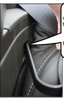
Now lower the wind deflector into the back seat area so the rear bracket goes into the slot beside the rear seat.
